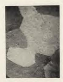
Fig. 23. (x 33 Diameters. Oblique Illumination.) Same as Fig. 22 after annealing at  $180^{\circ}$  C. for seven days.
